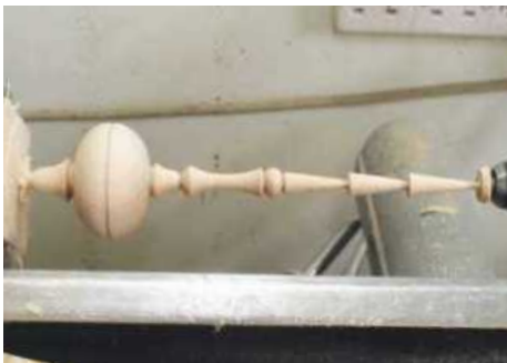
▲ Pic.7 Holding one end in the chuck means you only have to put very light pressure on the tailstock. The piece is very weak now so you have to be very careful in taking the top down
